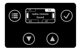
In the Remote submenu, the menu fields are replaced. At the top left, the channel (key on the hand-held transmitter) can be selected. At the bottom left, a new radio remote transmitter is taught-in and at the bottom right, the taught-in hand-held transmitters are deleted again.
