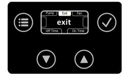
The waiting time can be set in minute increments at the bottom left. Similarly, the fogging time can be set in minute increments at the bottom right.
