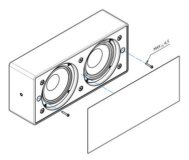
For this application, do not use screws with diameter greater than 4.5 mm.
